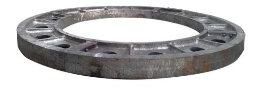
**PRODUCT:** Girth Gear **PROCESS:** Casting **APPLICATION:** Rotary Kilns, Ball Mills on Cement, Mining and Minerals Industry, Rotary Dryers, Pulp & Paper MATERIAL: ZG45, ZG42CrMO, GS34CrMo, 34CrNiMo6, GS34CrMo4 Carbon steel, alloy steel or according to customer's requirements.
