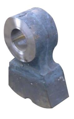
PRODUCT : Hammers PROCESS : Casting APPLICATION : Hammer crushers MATERIAL : Carbon Steel / Manganese Steel / NiHard IV / Bi-Metal / Double Heat Treated / Hardfacing Welded according to customers requirements. **PRODUCT :** Cone Crusher Parts, Spider,
